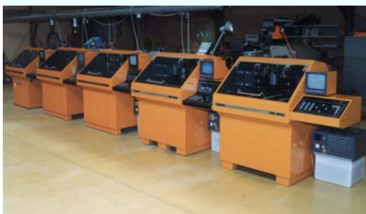
Flexibility: Mape machines can be run in parallel for mass-production or individually for low volume, flexible production.
